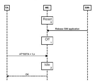
SAT starts in the RESET state when the module powers up. If the SIM application starts, SAT returns to the OFF state.
